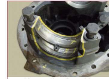
Adjustment Ring – Damaged Cups
